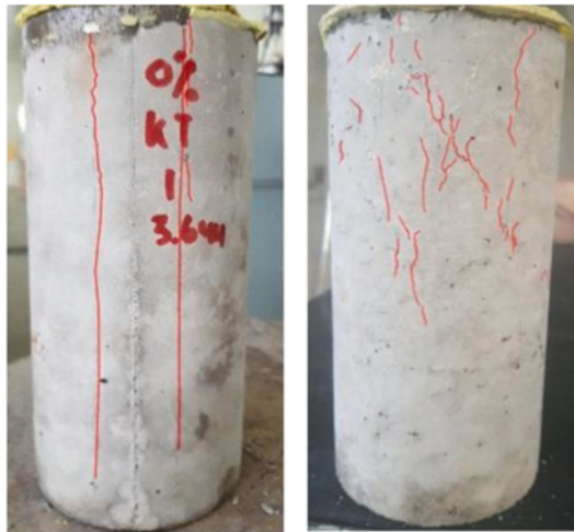
a. Normal concrete b. PET waste concrete
